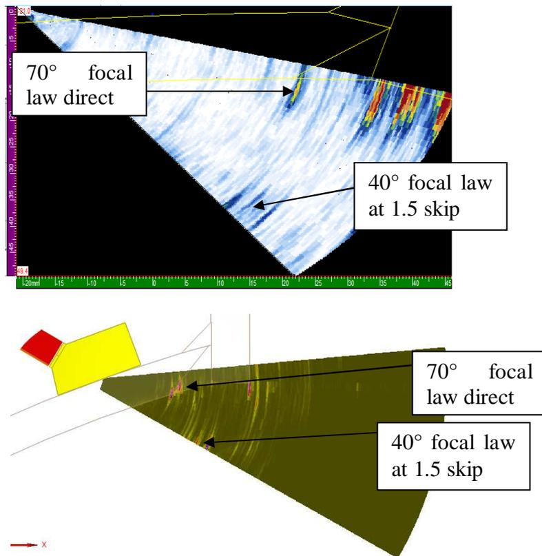
Figure 9 Perpendicular surface notch at 270°
