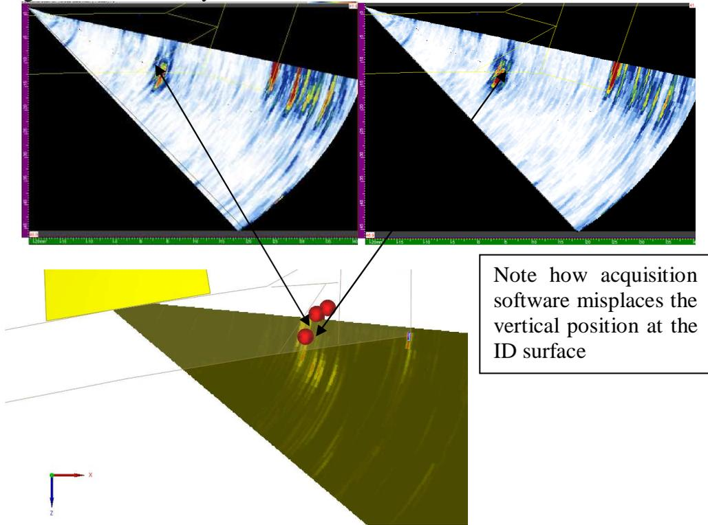
Figure 8 Angled Surface notch at 90°
