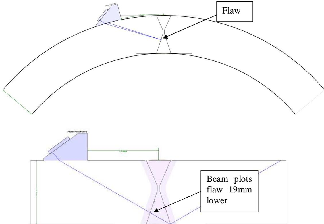
Some software is capable of geometric correction for skip on curved surfaces and can correctly place the indications with respect to the local weld geometry. Figure 14 is an image from the CIVA simulation software that uses the CAD geometry to plot the ray paths of each focal law and makes provision for the curvature.
