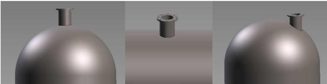
Ultrasonic inspection of nozzle welds is primarily done from the surface of the component where the weld bevel is made. Nozzle types can be identified as either “set-on” or “set-through” nozzles. Set-on nozzles have the secondary cylinders (i.e. the nozzle) prepared with the weld bevel, and set-through have the primary vessel prepared with the bevel. Examples of these two nozzle types are illustrated in Figure 2.
