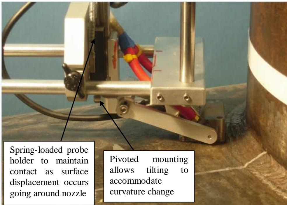
Volume coverage of the weld in the various positions, as the probe moves around the nozzle, can be estimated using popular software. Figure 4 illustrates the beam selections and probe details for the weld examination from the vessel OD for the mock-up used for this demonstration.
