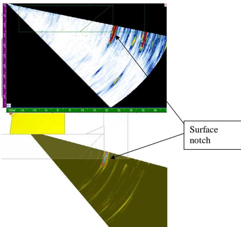
A polar plotted B-scan can be made with both the acquisition and CIVA modelling software. Figure 11 illustrates a close similarity of the detections in the polar plots. Only the cluster of porosity on the 325° position shows as weaker (this could be remedied by arranging pores with sufficient density to duplicate the same conditions).
