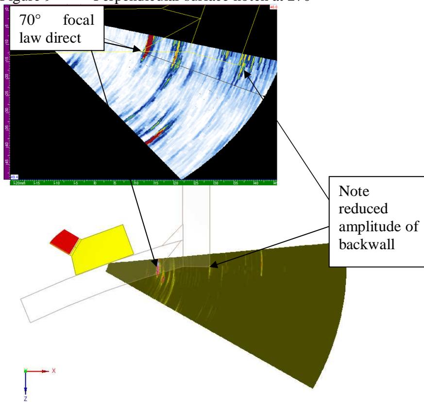
Figure 10 Surface notch at 180°
